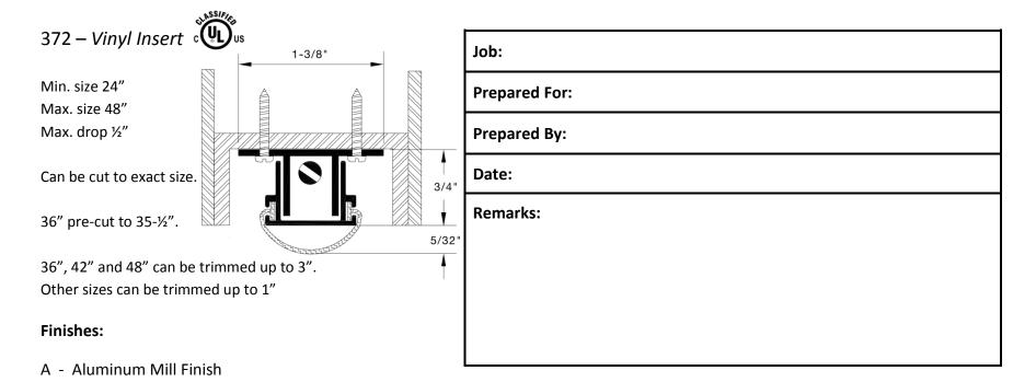
Note: Door bottoms are not designed to seal directly on carpet. For best results door bottoms should seal on a solid surface. The solid surface should be positioned above the level of the floor covering on either side of the door. Door bottoms are field reversible and can be used in semi-mortised applications.
